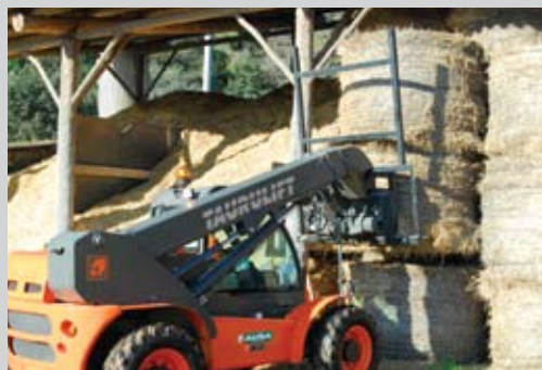
Forks with side shift with Multi-Tach system
